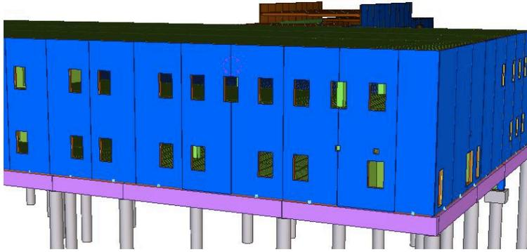
and MEP components, all with a precast concrete system as the superstructure of the buildings. Schwab Structural Engineering, Inc. utilized TEKLA in developing the precast superstructure which was then integrated into the overall REVIT BIM model prepared by lead architect/engineer PBS&J. Design assistance was provided by the
