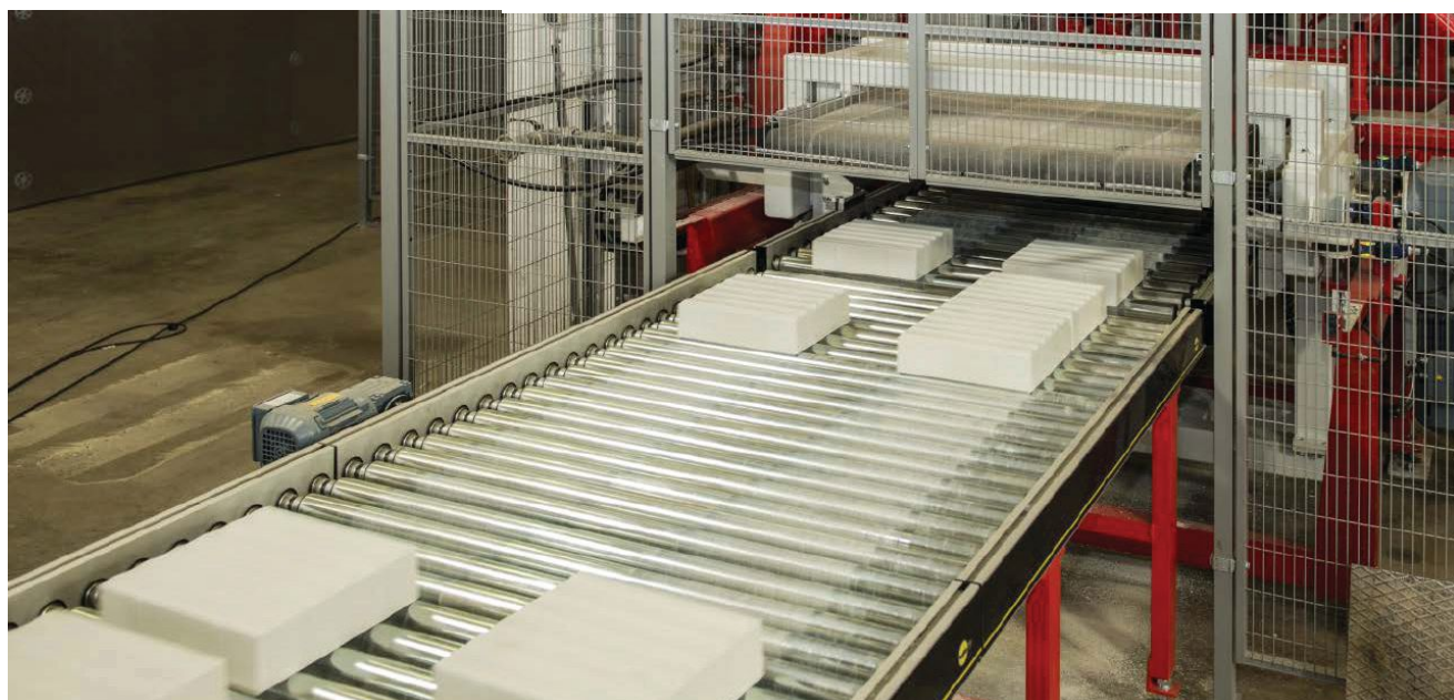
BFS vibration technology underpins the Prima Scape program for automated hardscape slab and veneer stone unit production.
